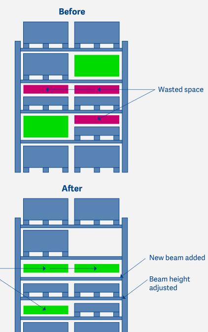
Optimized spacing because of adjusted beam
